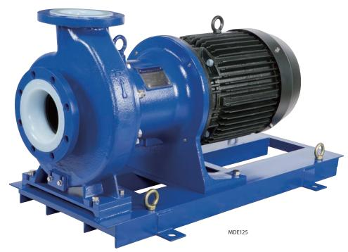
The MDE Series comprises the world's largest-class non-metalic magnetic drive pumps for chemical processing, with a maximum delivery of 4.0m³/min. and a maximum head of over 70 meters. The liquid end parts, plastics are made of advanced corrosion-resistant materials such as fluororesins and fine ceramics, and the major fluoroplastic-made parts are reinforced with special metal inserts for added mechanical strength and durability.
