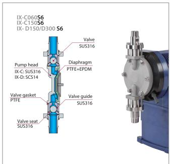
Note: EPDM of PPS and the diaphragm of the pump head is not wetted.
